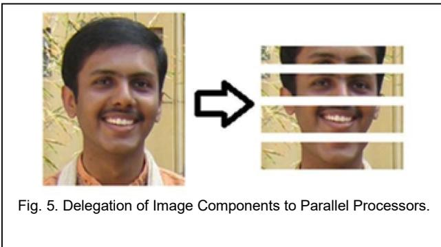
Fig. 5. Delegation of Image Components to Parallel Processors.
