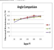
The procedure is carried out in a similar fashion than that of fill ratio. The thermal resistance of heat pipe is filled with R-32 at various inclinations. The thermal resistance of the thermosyphon is depicted by (R) and Te and Tc are average values of temperatures at the evaporator and condenser sections respectively and Q is the heat supplied to the heat pipe
