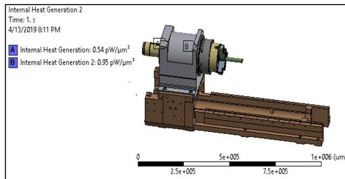
**Fig.13 Numerical Model for Thermal Behaviour in Lathe Bed**
