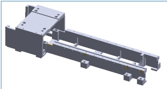
**Figure 1 Steel Reinforcement of the Polymer Composite Lathe Bed**
