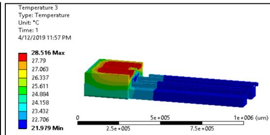
**Fig.16 Temperature Distribution in Proposed Lathe Bed after Coolant Passage**
