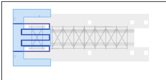
**Fig.15 Coolant Pipe Design in Proposed Design**
