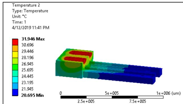
**Fig.14 Temperature Distribution in Proposed Design Lathe Bed**
