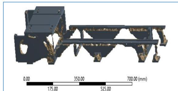
**Figure 2 Optimized Structure of the Existing Steel Reinforcement**
