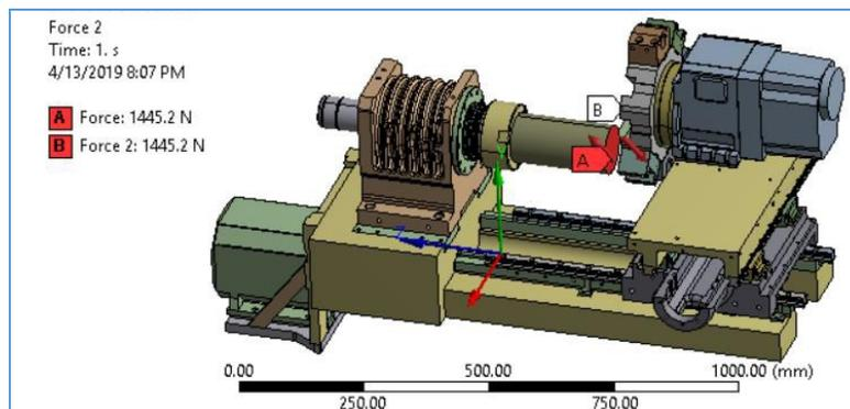
**Figure 3. Forces Acting on the Lathe Assembly**
