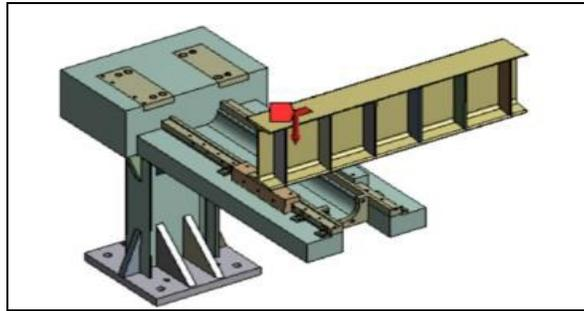
**Figure 12. Numerical Model for the Test of Bending Stiffness**
