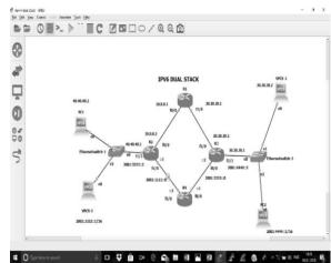
Figure 4 Dual Stack -Dynamic Routing Network
