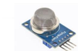
An alcohol sensor detects the attentiveness of alcohol gas in the air and an analog voltage is an output reading. The sensor can activate at temperatures ranging from -10 to 50° C with a power
